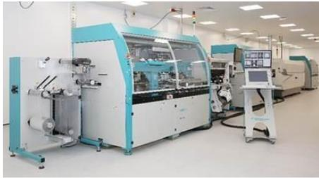
also demonstrating the assembly of hybrid large area printed electronics including assembly from wafer. Further it showed the capability for very high speed printing of conductive ink applications onto a range of substrates from Paper to PET.
